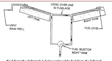
Fuel from the right tank is being replaced by fuel from the left tank
