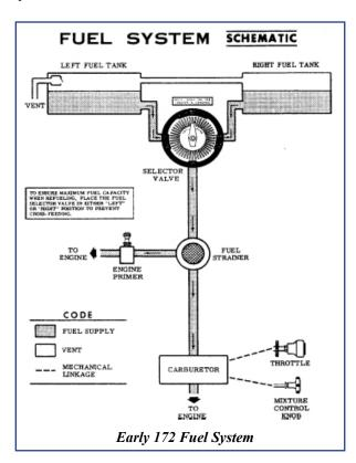
have the same head pressure then the tank with the lower head pressure will flow the slowest.
